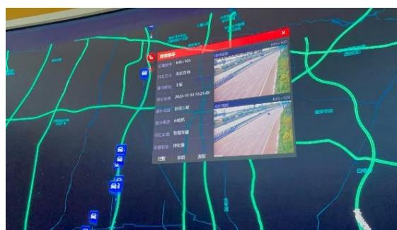
Automatic detection of stopped vehicles
